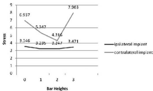
**FIGURE 7.** Maximum stress values for ipsilateral and contralateral fixtures according to the different bar heights. Though contralateral values are in the minuses, they are illustrated above the X-axis for the ease of comparison and also to save space.
