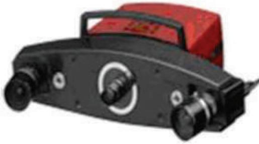
**FIGURE 1.** Noncontact measuring device (ATOS II).
